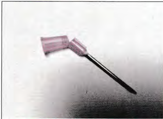
Figure 3- Cracked Hub (Worst Case)
