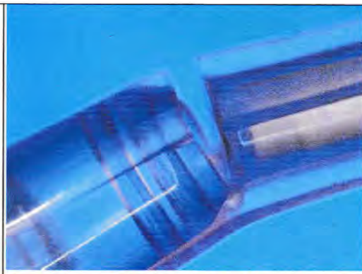
Figure 4- Cracked Hub (Worst Case)
